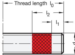
$l_1 \approx 2 \text{ to } 3 \times \text{Thread pitch}$
